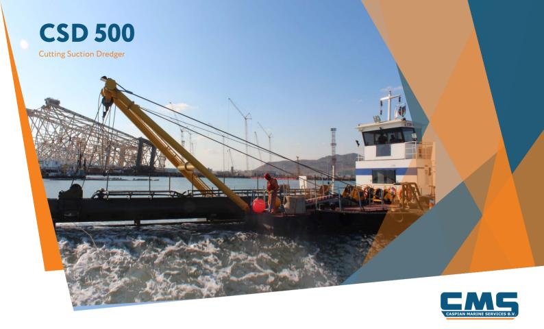
The Cutter Suction Dredger CSD500 may be used only to transfer mud, sand, gravel and or water mixtures or other similar materials.
